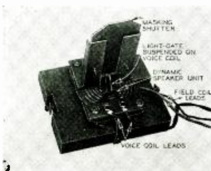
Fig. A Photograph of "light gate."
